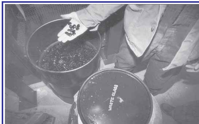
Vitrification Glass used to stabilize nuclear waste
